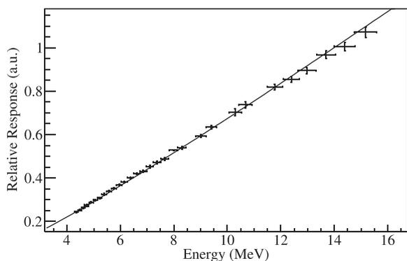
FIG. 3. The data points represent the relative light yield of the 0.5% stilbene-doped bibenzyl mixed single-crystal organic scintillator as a function of proton energy deposited in MeV. The energy bin width varies via a non-linear transformation using 4 ns time bins. The line represents a fit to the data using Birks' semi-empirical relation for the number of scintillation photons generated as a function of proton energy deposited.
