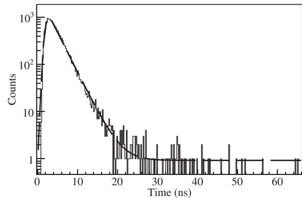
FIG. 1. Time dependence of intensity of scintillation light from a 0.5% stilbene-doped bibenzyl mixed single-crystal organic scintillator. The dashed line represents a fit to the data using a single component exponential decay convolved with a Gaussian distribution.
