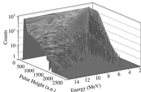
FIG. 2. Two-dimensional surface plot of pulse height in arbitrary units versus neutron energy in MeV. The ridge at 4 MeV corresponds to high energy neutrons produced from the following cyclotron beam pulse.
