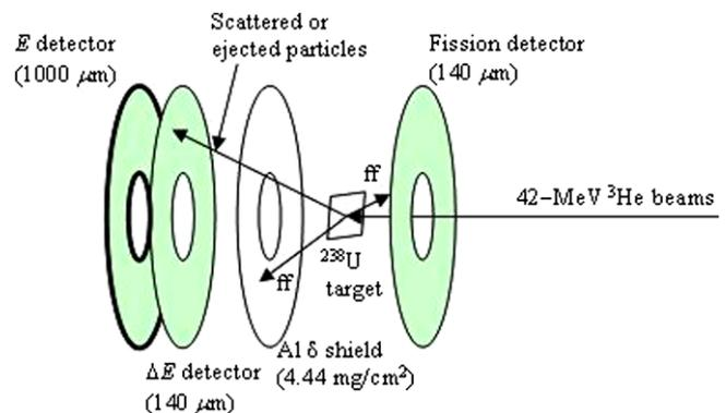
Fig. 1. Experimental setup of  $^{238}\text{U}$  target, silicon telescope ( $\Delta E + E$ ), Al shield, and fission detector. Arbitrary directions for the scattered/ejected particle and fission fragment (ff) along with the incoming beam on the  $^{238}\text{U}$  target are shown.
