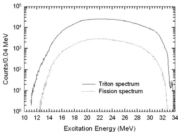
**Fig. 3.** Integrated singles triton spectrum and background-corrected fission spectrum of the particle telescope and fission detector.
