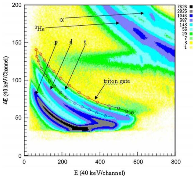
**Fig. 2.**  $\Delta E$  vs.  $E$  plot for a single ring at  $49^\circ$  with respect to the beam axis shows different ejected particles from the interaction of 42 MeV  $^3\text{He}$  beams with the  $^{238}\text{U}$  target. Protons ( $p$ ), deuterons ( $d$ ), and tritons ( $t$ ) are located in the lower left side in the plot and part of the  $^3\text{He}$  and  $\alpha$  particles are visible in the upper right corner in the plot. A typical triton gate is shown.
